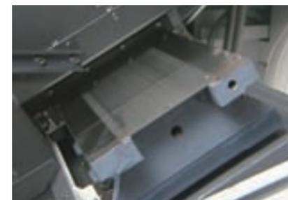
Box way slide for long term operation with and high reliability. The bearing rigidity has been improved by up to 140% with the design upgrade to 3 rows of X-axis support bearings. More stable machining for a long term and heavy duty cutting is possible.
