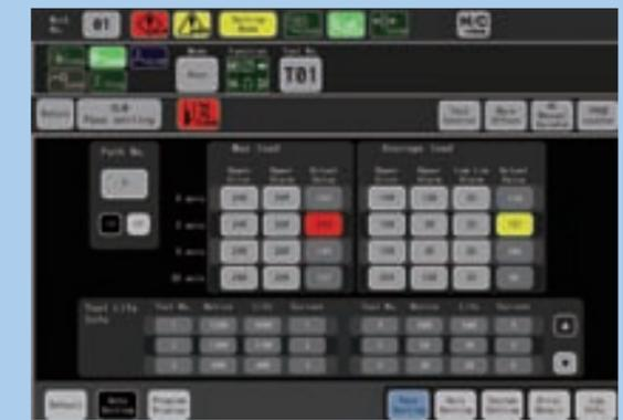
Abnormal loads due to tool damage during machining can be detected. It is possible to specify threshold values by referring to the maximum load and average load based on each cutting path instance displayed on the screen.
